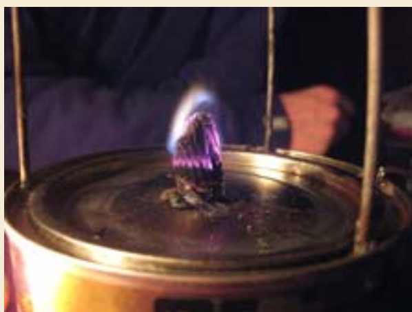
Illustration 4.3: Jatropha oil lamps are not used because they are not working properly.
