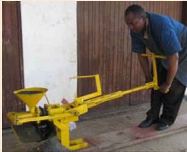
Illustration 6.13: Demonstration of ram press operating techniques at CAMARTEC.
